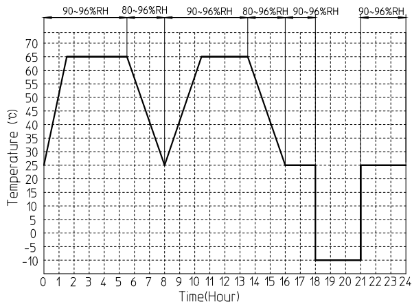
Fig 1. Temp. and Humidity Cycle
