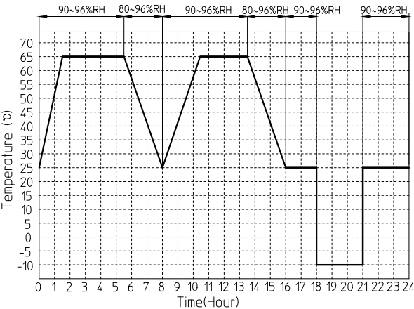
Fig 1. Temp. and Humidity Cycle
